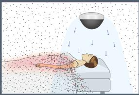
Temperaturecontrolled Laminar Airflow (TLA) filters the air in the breathing zone and removes 99.5% of all allergen and irritating particles larger than 0.5 µm.
