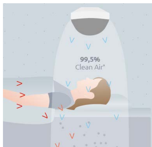
Figure 2b: TLA-generated laminar air flow enveloping the breathing zone
